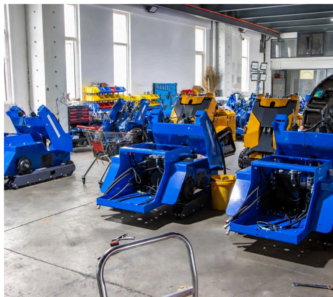
Painted frames on the assembly floor.
