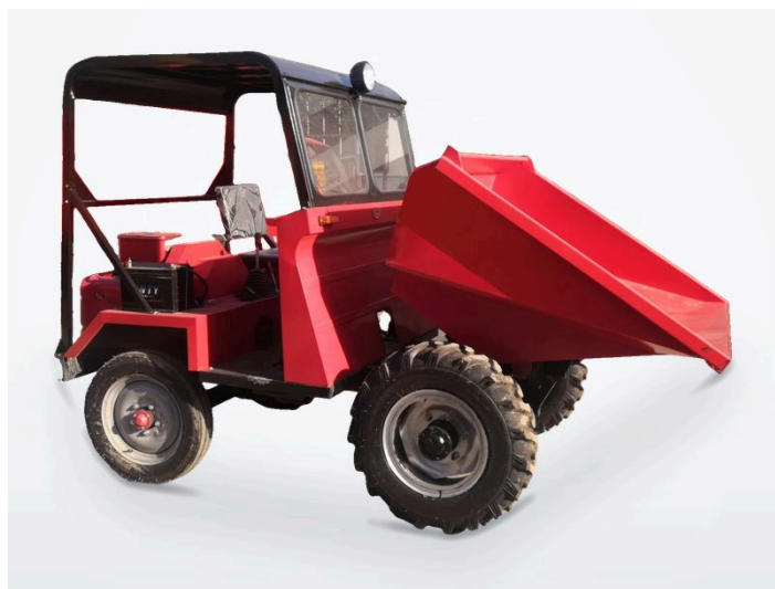
FY15, hopper tipped forward.
