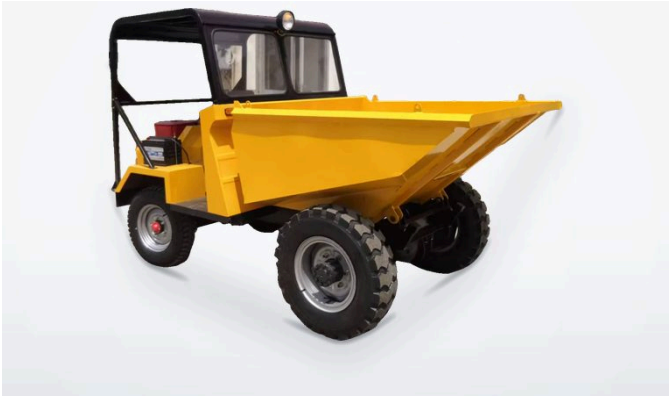
Front-tip hopper, larger front tyres
