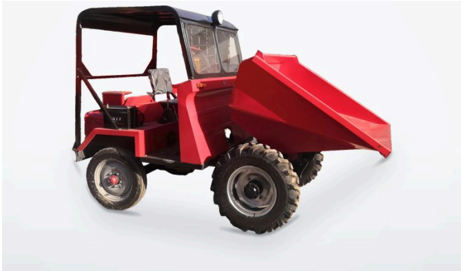
Hopper tipped forward
